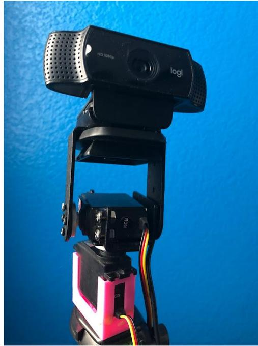
Fig. C1. Servo Stand with Tripod [42]
