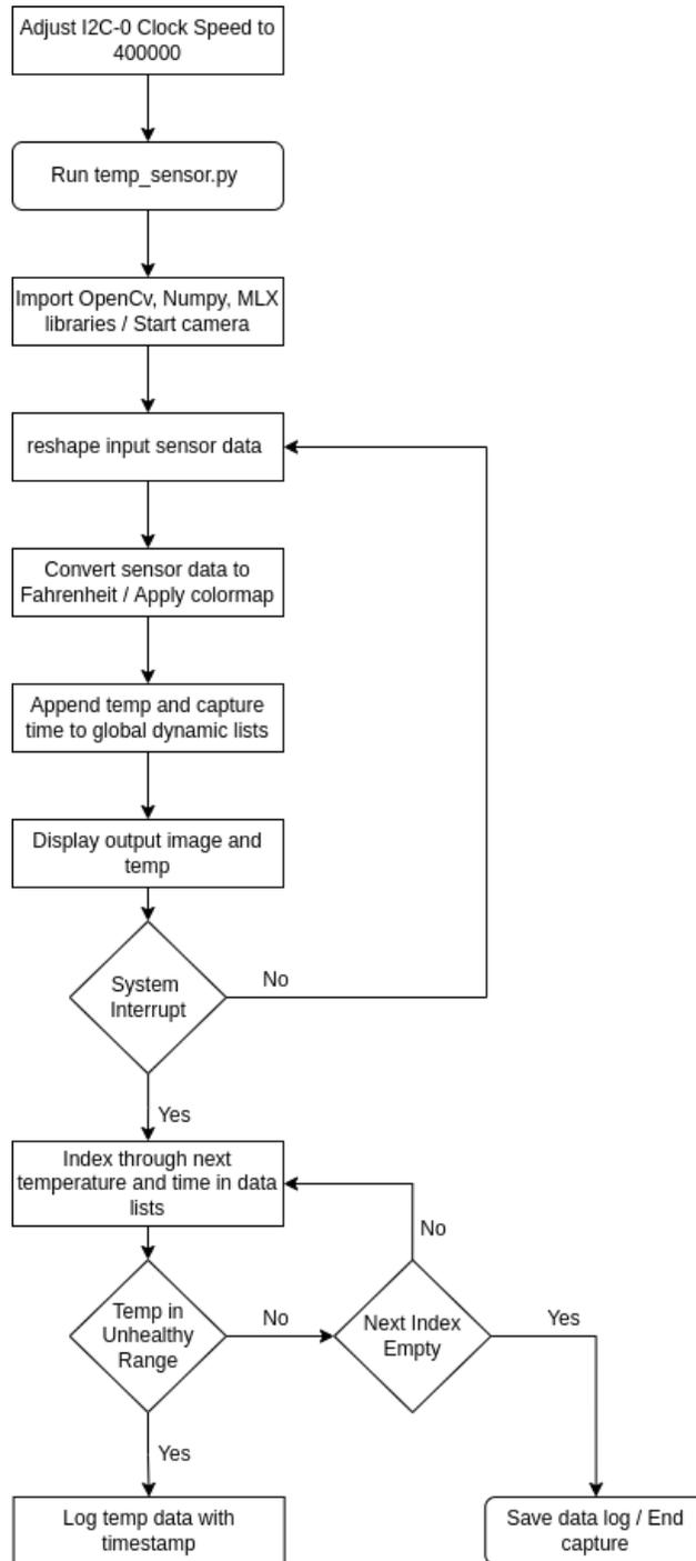
Fig. B3. Temperature Sensor Software Flowchart [41]
